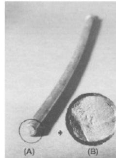
FIGURE 12.3.4 The smooth part of a 316L stainless steel Harrington spinal distraction rod that fractured by fatigue in vivo . Note the bend in the rod (the rod was originally straight) and (insert) the relationship of the crack initiation zone of the fracture surface to the bend. The inserted photo shows the nature of the fatigue fracture surface, which is characterized by a region of "beach marks" and a region of sudden overload failure. (Photo courtesy of Brunski, J. B., Hill, D. C. & Moskowitz, A. (1983). Stresses in a Harrington distraction rod: Their origin and relationship to fatigue fractures in vivo . J. Biomed. Eng. , 105, 101-107.)
